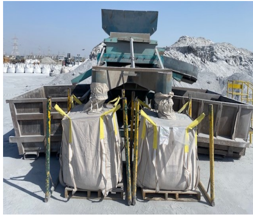
Figure 6. Fine material output from segregation machine (< 0.8 mm).
