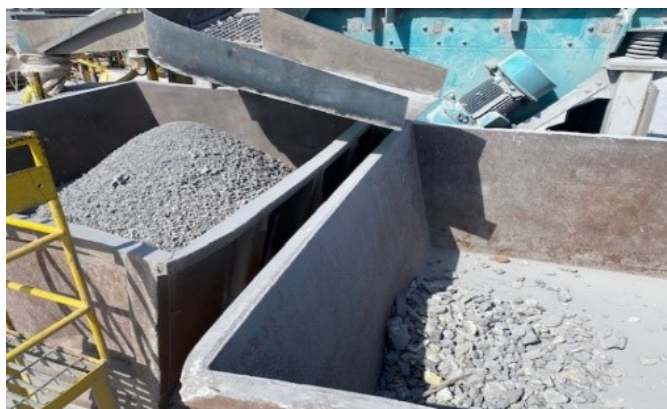
Figure 8. Scrap material output from screening process (> 25 mm).
